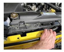
Once all six pins are removed, pull the grill slightly forward. (Figure 1) From the bottom of the grill, pull until the snap clips come out and release the grill. (Figure 2)
