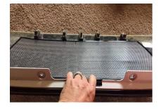
Reinstall the grill onto the Jeep starting with the bottom snap clips first. Slide the insert in between the grill and the radiator. The insert will rest on the clips at the bottom interior of the grill itself. Reinstall the top push six pins.
