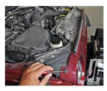
Use a screwdriver to pry up the pins. Once lifted, they can be removed by hand or with a pair of plyers.
