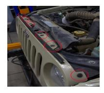
Under the hood, there are six pins that will need to be pulled to install the insert. Same for JK and JL
